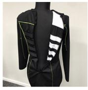
The white straps on the inside of the dress consists of pockets to place actuators that then can convey signals to the users as haptic signals displayed on the back in a matrix setup.
