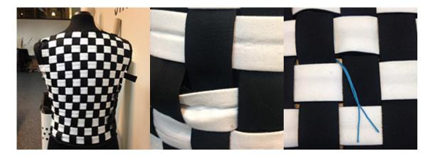
The back of the vest consists of straps in a plain weave construction, providing a great freedom in placement of actuators.
