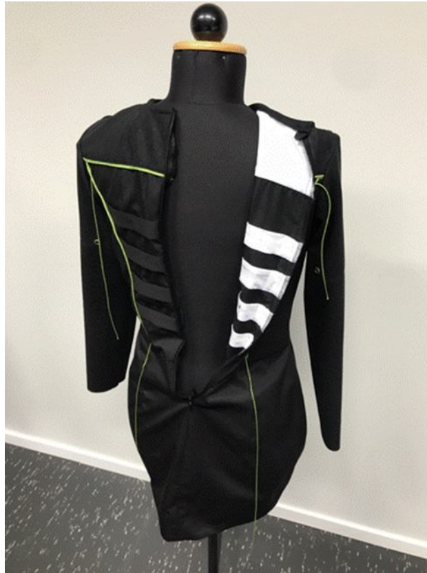
Figure 13. The Black dress developed within the SUITCEYES project by HB. On the inside of the back there is matrix (white lining) of 4 by 4 pockets where coin vibrators can be placed. Vertical symmetric in this matrix there is the back zipper that gives access to the vibrators as well as enabling taking it on and having a close fit. Green parts are a developed seaming technique for housing electrical conductors for powering and signal control.
