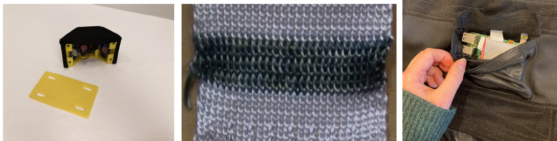
Figure 9. Examples illustrating different integration strategies a) integration only using a back plane and screws enabling stability for a sensor (black) that is to be in a certain angle b) integration in using conductive tread knitted together with ordinary polyester; c) integration off by using a communicative (Raspberry Pi unit) for which the garment becomes connected to the outside for both outward and inward communication.
