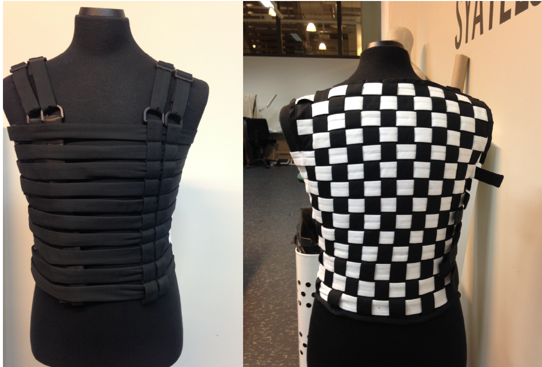
Figure 16. The Chessboard Dress developed within SUITCEYES project by HB. This is in principle more of a psychophysical testing device than a full-fledged consumer product. It addresses the problem of the need to positioning vibrators at a certain body location but having a garment that fits different body sizes. It is here solved by making a kind of weave construction with warp and weft “tails”. Behind each of the crossing points seen a coin vibrator could be inserted which then actuate on the skin side. Tails in the weft direction are having a strap function tightening up the
