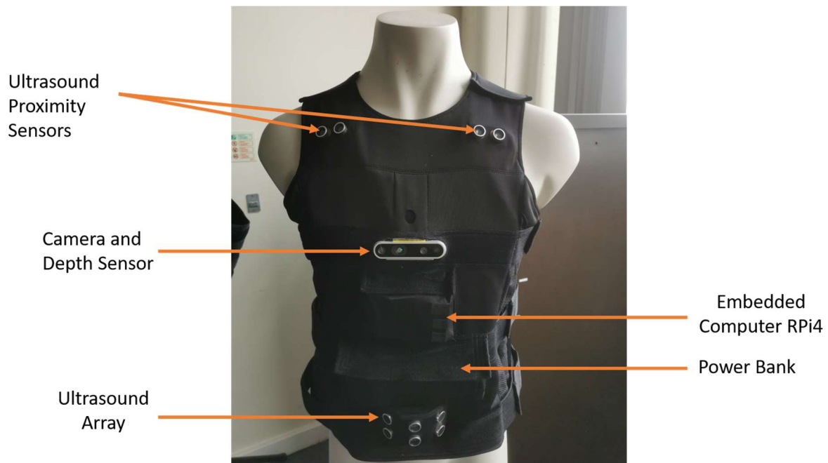
Figure 13: Current prototype of the HIPI system with all components mounted.
