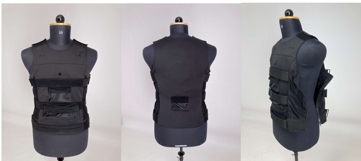
Figure 7: Prototype Garment showing front pockets for power pack (lower) and Raspberry Pi (upper); back pocket for motor driver boards; and side opening zip.
